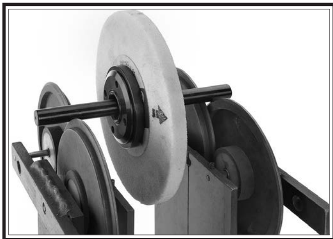
Figure 39. Wheel on balancing fixture.
