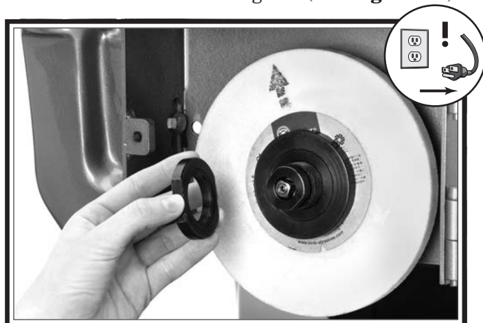
Figure 24. Exposing wheel retaining washer.
