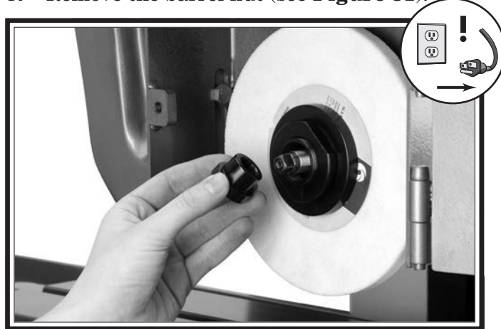
Figure 31. Barrel nut removal.
