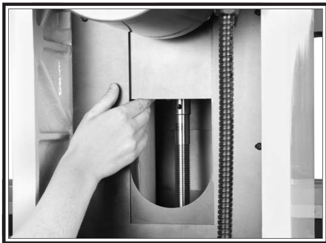
Figure 46. Upper leadscrew inspection.
