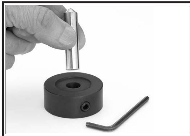
Figure 38. Dressing tool setup.
