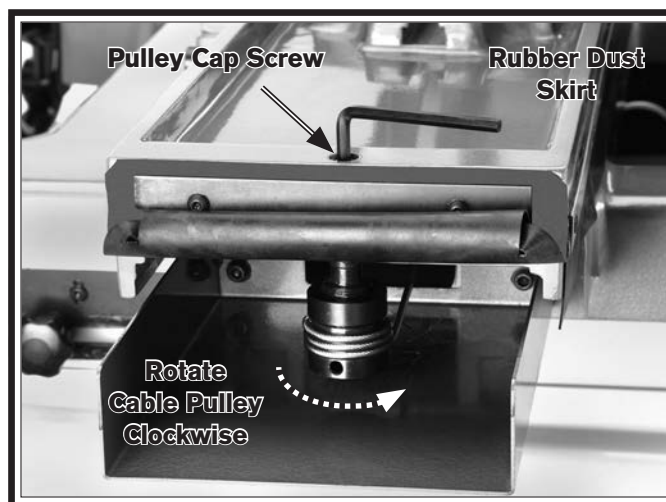
Figure 49. Adjusting cable pulley.
