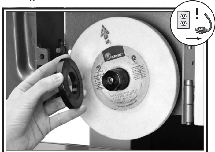
Figure 25. Wheel ready for removal.
