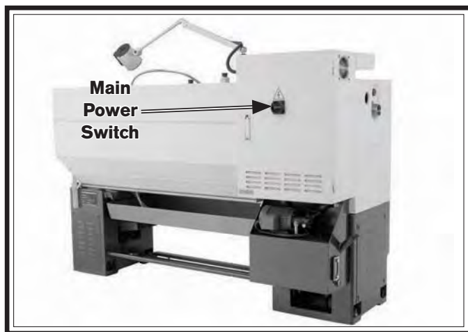
Figure 33. Main power switch.
