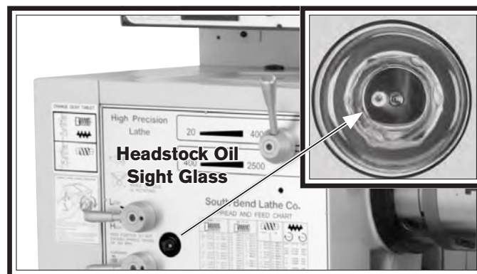
Figure 109. Location of the headstock oil sight glass.
