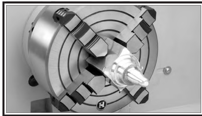
Figure 54. Example of non-concentric workpiece correctly mounted on the 4-jaw chuck.
