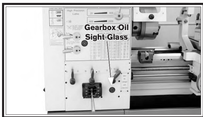
Figure 112. Gearbox sight glass location.
